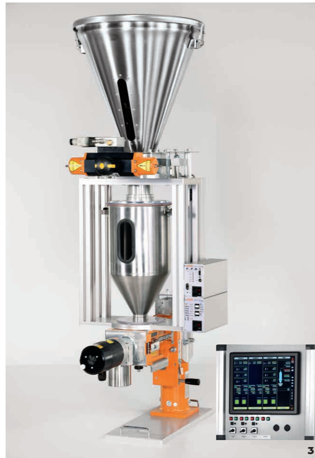
3 PLASTICOLOR single gravimetric dosing unit with weighing hopper, PPM Module with function front for the basic configuration (calibration, taring, change of screw/cylinder, quantity test, etc.), with additional PPM Interface . Operation via Bus connection to customer's PLC or the PLASTICOLOR IPC with PPM Touch Screen Control .
