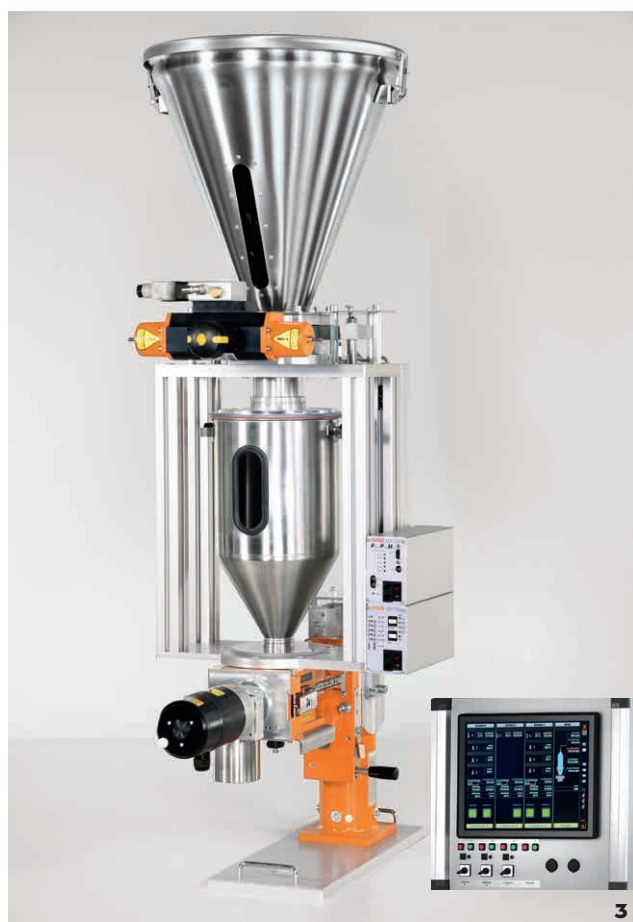
3 PLASTICOLOR single gravimetric dosing unit with weighing hopper, PPM Module with function front for the basic configuration (calibration, taring, change of screw/cylinder, quantity test, etc.), with additional PPM Interface . Operation via Bus connection to customer's PLC or the PLASTICOLOR IPC with PPM Touch Screen Control .
