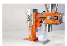
Taking a sample via the neckpiece slide
